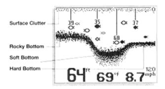
Sonar targets which are not physically attached to the bottom may take one of many shapes. Surface clutter is the layer of water near the surface which is rich in algae and other growth, and often is aerated by wind or wave action. This area interferes with sonar transmission and often appears on-screen as regular clusters of individual dots near the "O" line.
